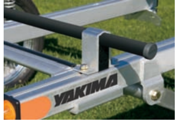
Position Block with Square Bar on top. Slip Tower over T-Bolts. Attach washers and nuts.
