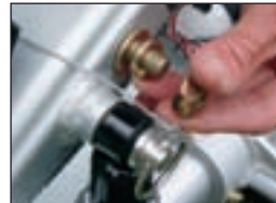
7D Flat washer, lock washer, nut
