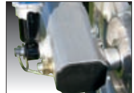
7E Tighten to 57 ft. lbs., right Wheel Block shown
